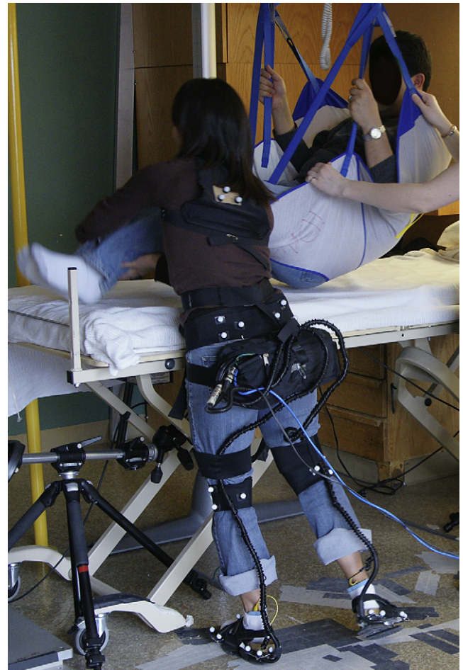
Fig. 1. Subject performing the Legs Down activity in the 'secondary' condition using a floor lift.
